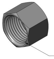
3/8 NPT PIPE SIZE, 18 THREADS PER INCH, 0.43" THREAD ENGAGEMENT
